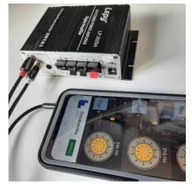
This picture shows the correct RCA cable connection between the amplifier and the phone.
