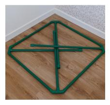
Connect the 4 pieces of pipe with external couplings into the slip tee in the middle of each Corner Assembly and let them lie down flat on the ground. It is easier if you insert pipes into two opposing corners first. Note - If you purchased a 3ft mini-pyramid, skip to Step 4.
