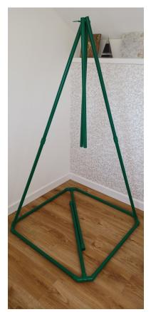
NOTE - WHILE PERFORMING STEPS 4 AND 5, DO NOT PUSH THE PIECES OF THE TOP ASSEMBLY TIGHTLY INTO THE EXTERNAL COUPLING AT THIS TIME. ONLY APPLY ENOUGH PRESSURE TO KEEP THEM FROM FALLING APART. WE WILL TIGHTEN THESE CONNECTIONS LATER AFTER POSITIONING THE TOP ASSEMBLY AND TIGHTENING THE ZIP-TIE (Step 6).
