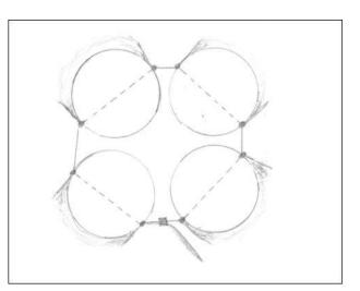
Once the pipes are in their proper position, slowly pull on the zip-tie to tighten it until the four vertical pieces are touching each other at the top. Cut off the remaining piece of the zip-tie with scissors.
